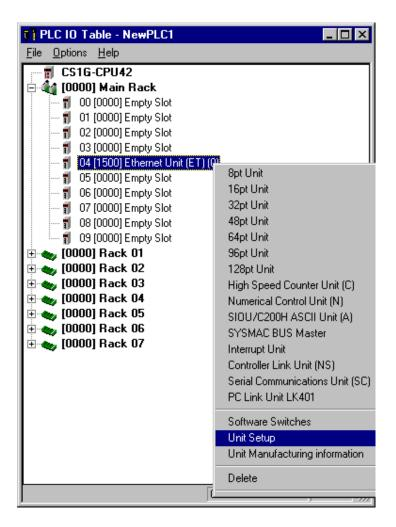
Click "Unit Setup". The "Ethernet Unit CPU Bus Unit" dialog box appears:
